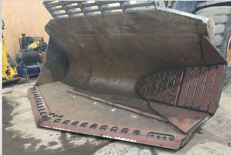
Finished bucket with welded wear plates
